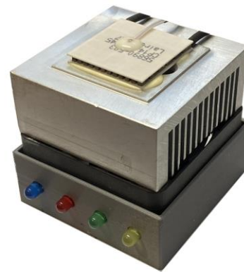
Fig. 3. Heat sink with TEM, thermistor, fan, and base with LEDs.
