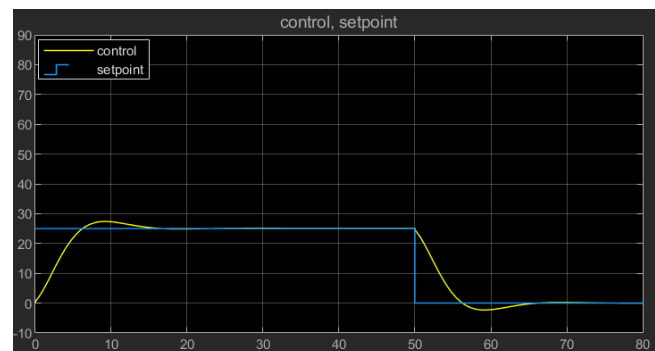
Fig. 13. Step response from 25.0° C to 0.0° C.
